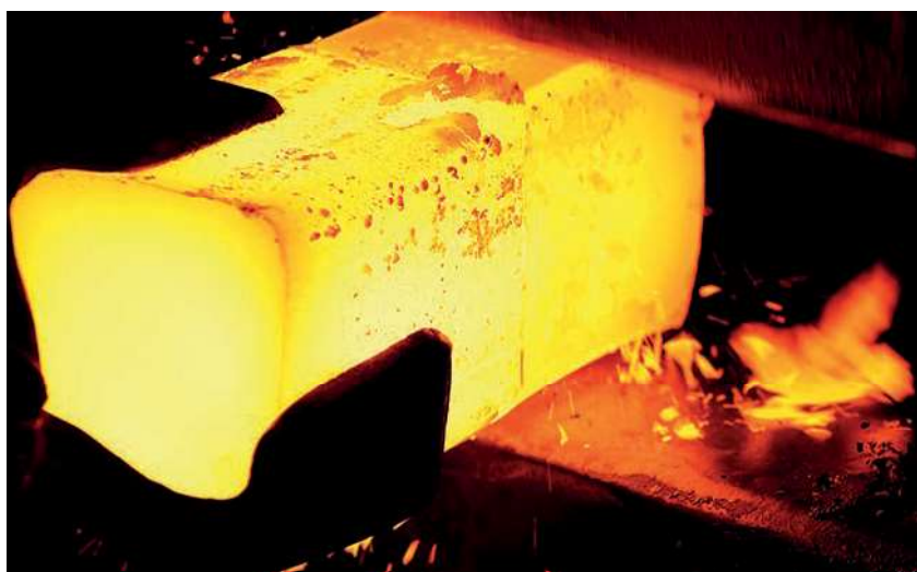
Square billets (edge length 50 to 120 mm) or round bar material (18.5 to 200 mm in diameter) can be used as raw material.
