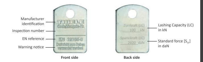
Tags as per DIN EN 12195-3 show on their front the number of the standard specification, the name of the chain manufacturer, the inspection number, as well as a warning that the chain must not be used for lifting. On the back side of the tag the maximum permissible lashing capacity (LC) in kN and standard tensioning force  $(S_{TF})$  in daN is hard-stamped.
