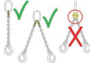
If two chain legs are assembled into one connecting link half for alternate use of the legs, only one chain leg must be subjected to loads!
