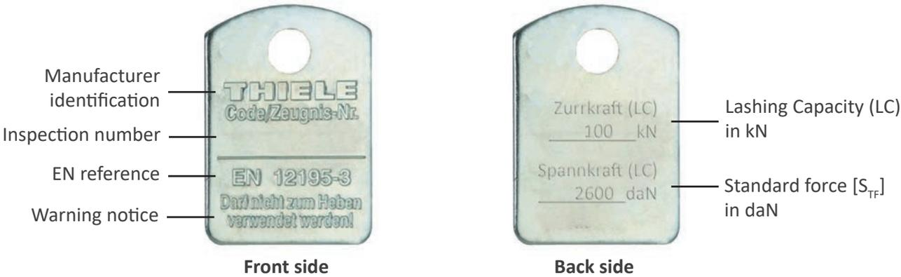
Tags as per DIN EN 12195-3 show on their front the number of the standard specification, the name of the chain manufacturer, the inspection number, as well as a warning that the chain must not be used for lifting. On the back side of the tag the maximum permissible lashing capacity (LC) in kN and standard tensioning force (S<sub>TF</sub>) in daN is hard-stamped.
