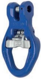
The Grade 100 skip suspension links TWN 1869 connect chain slings with the pivots on containers, e.g. containers according to DIN EN 30720. The shape of the eyelet is designed to fit container suspension pivots. The clevis design enables the direct attachment to the chain. The forged safety latch enables a one-hand operation. The manufacturing and testing requirements correspond to the ISO 8539 and DIN EN 1677-1, under consideration of Grade 100 working load limits.
